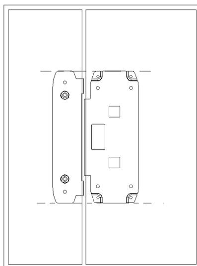
■ After the fixed bottom plate is aligned, close the screw on the side of the lock body and remove the rear panel. There is a cable connection between the front panel and the rear panel of the main lock, and the cable can be disassembled:
