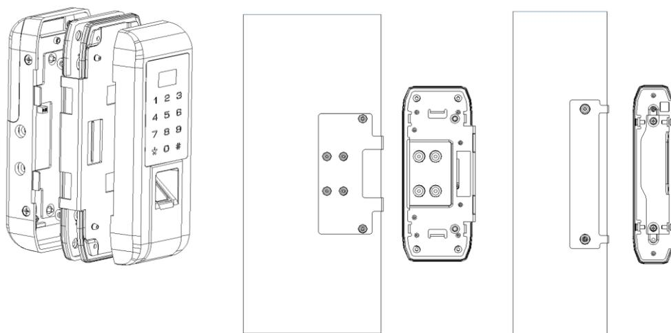
Note: When unscrewing the screw, hold the rear panel with your hand, and then remove the rear panel and then remove the rear panel.
