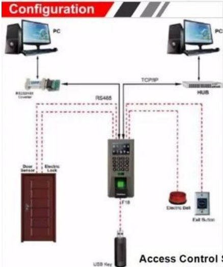
Access Control System Application Diagram
