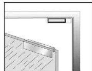
UL bracket installation
