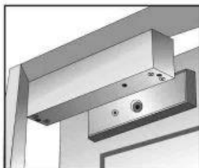
Amature plate installation
