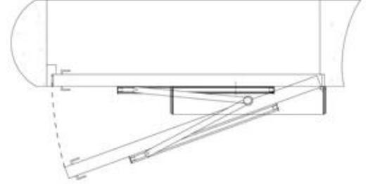
Push Arm Installation: Suitable for door wing opening outward (drive system inside)
