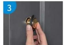
3 First place the front lock head into the decorative ring, and then insert both into the circular hole together
