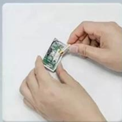
② install 23A 12V battery
