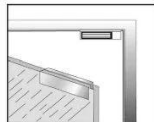
UL bracket installation
