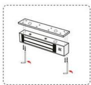
3. Separate the lock body and the the connecting plate with a hexagonal key.
