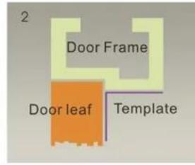
2 Close the door first, then place the upper side of template on door frame, while adjust the left side next to the door leaf.
