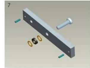
7 Make a combination based on the picture (add washer accordingly). The rubber ring must be added.
