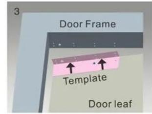
3 Mark screw positions of armature plate and magnetic lock on door leaf and door frame respectively.
