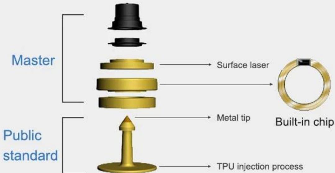
Note: The male standard has a pointed tip and the female standard has holes.
