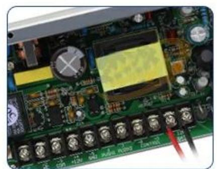
Ordinary access control power supply provides 1.5-1.8A current output, 208K 5A access control power supply provides 5A current output
