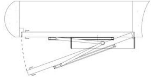
Push Arm Installation: Suitable for door wing opening outward (drive system inside)
