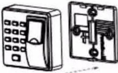
4. Install the machine on the fixed back cover.
