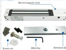
Remark: Please don't fix the screw of armature plate tightly. Let the rubber ring maintain proper elasticity.
