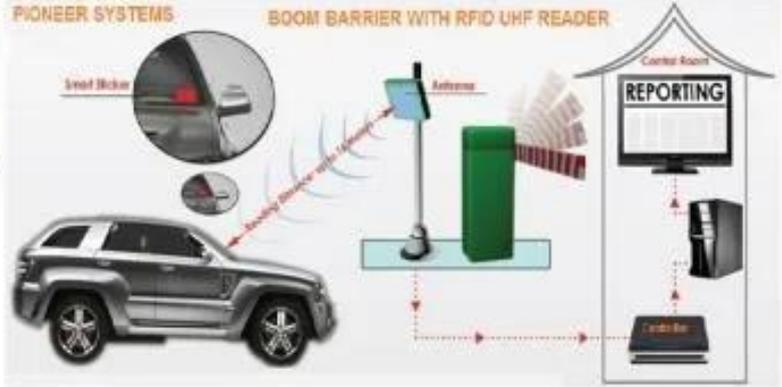
The diagram illustrates the system's workflow: a car with a 'Smart Sticker' on its windshield passes through a boom barrier equipped with an 'Antenna' (UHF reader). The reader communicates with the sticker and sends data to a 'Control Room' which displays 'REPORTING' on a monitor and prints a receipt on a printer.
