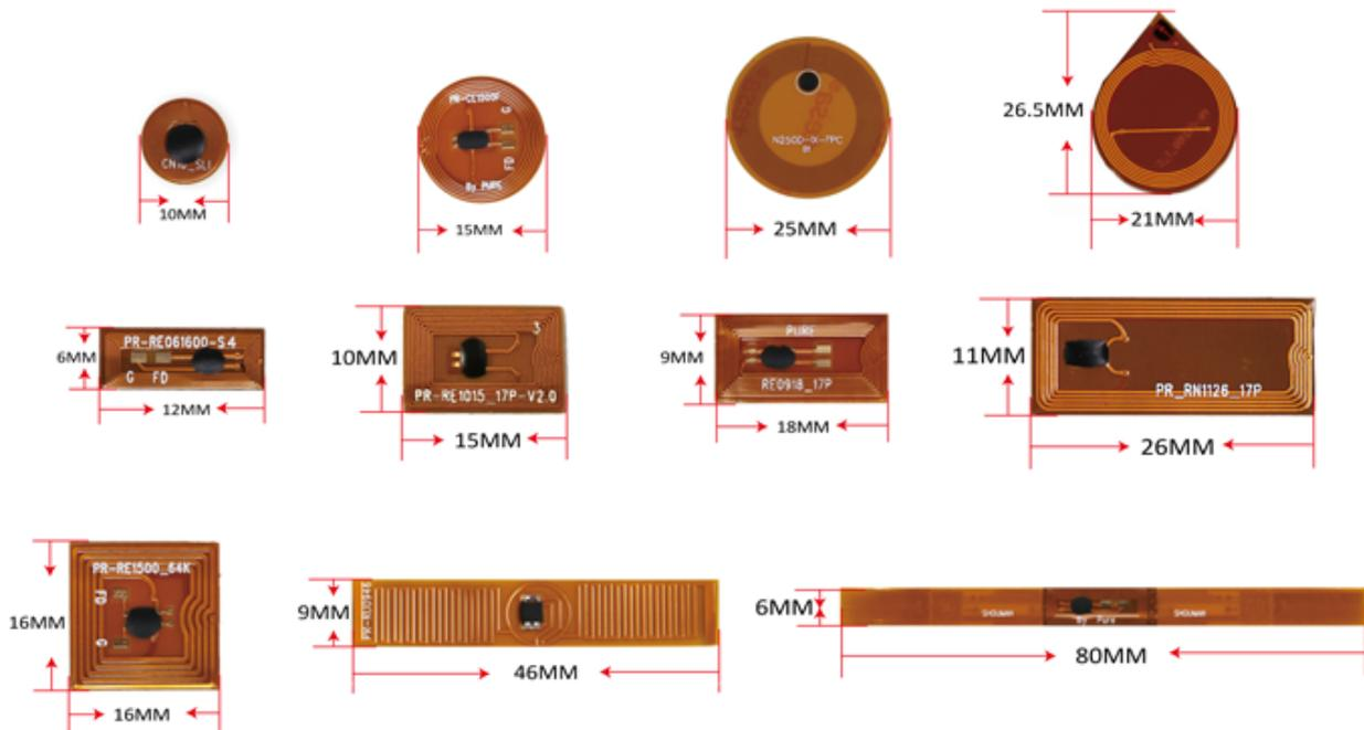
Flexible circuit board (Flexible PCB): Referred to as "flexible board", FPCB features: Can add anti-metal layer and adhesive, suitable for bending and use, light and thin, foldable, small pitch, multi-pin, small volume, high integration, multi-contact, etc. It is suitable for the design of custom labels, including special requirements for the shape.
