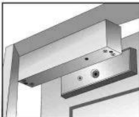
Amature plate installation
