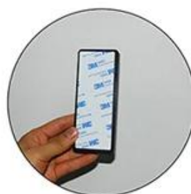
Stick it on the back of the keypad
