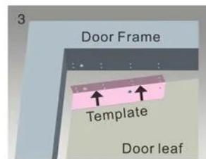
3 Mark screw positions of armature plate and magnetic lock on door leaf and door frame respectively.
