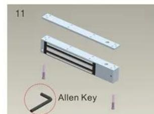
11 Use Allen key to screw the lock body on the mounting plate.
