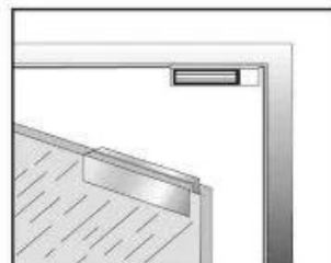
UL bracket installation
