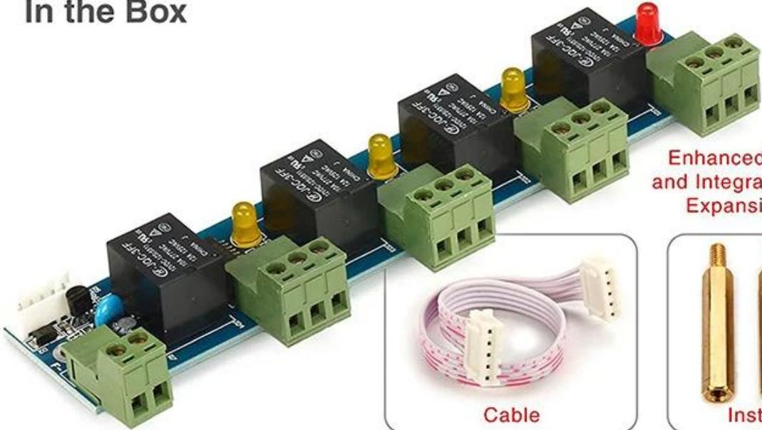
Enhanced Alarm Output and Integrated Fire Control Expansion Controller
