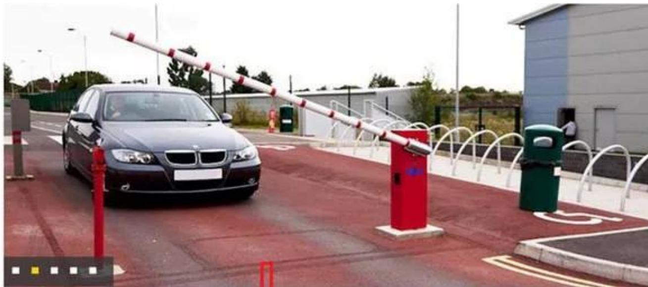
Single channel / dual channel vehicle loop detector with automatic barrier gates used for Vehicle access control
