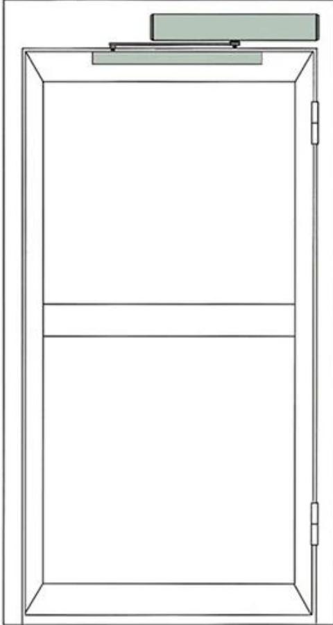
Push Arm Installation: Suitable for door wing opening outward (drive system inside)
