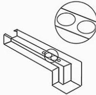
3. Use a hole opener to open the lock hole
