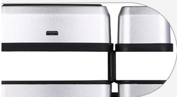
Emergency charging port
