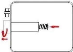
Factory default is inward opening. Push the bar of deadbolt and turn 180 degree to make it for outward opening.
