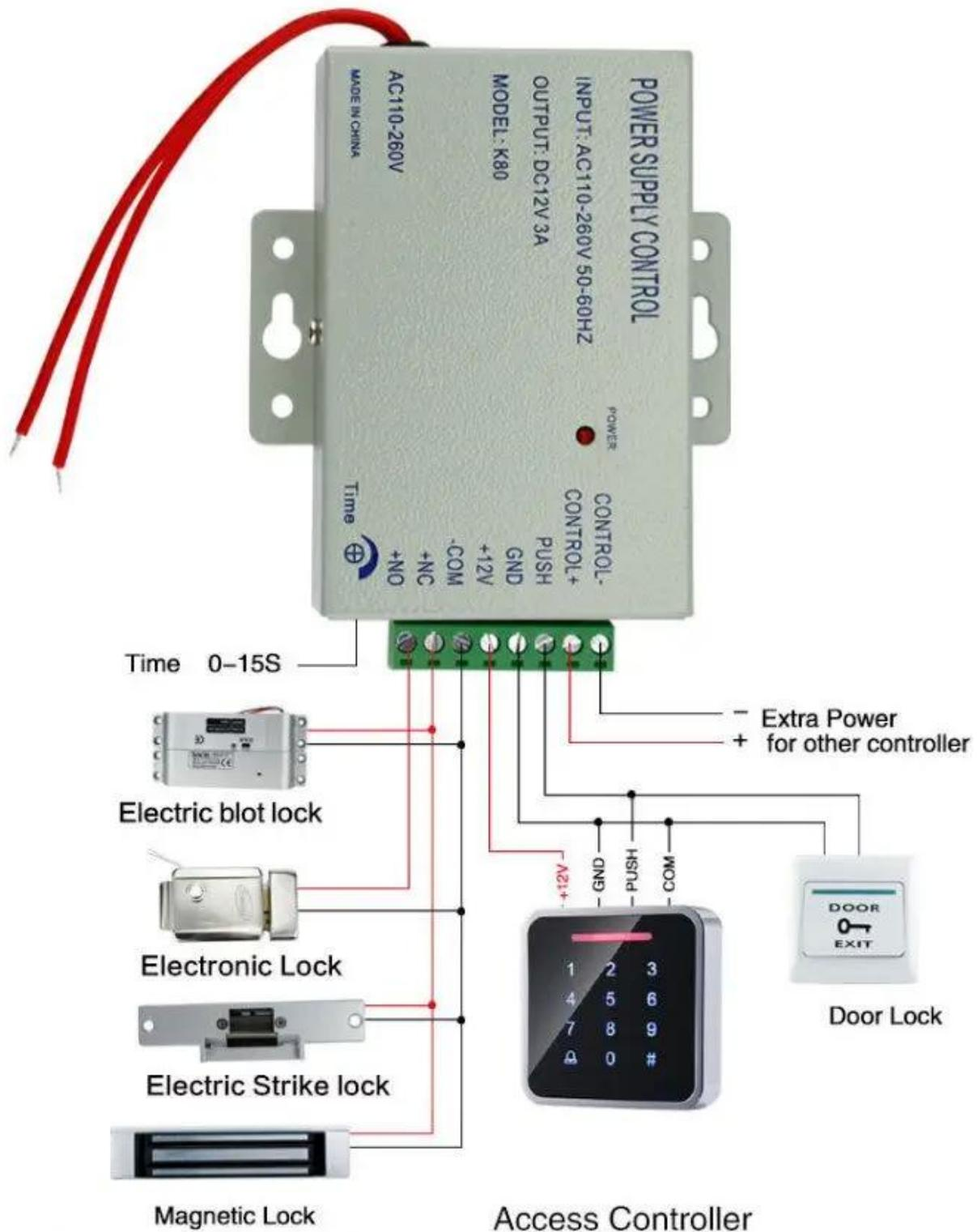
Attention when electronically controlled lock must be transferred to 0 seconds delay, to prevent burning of electric lock.
