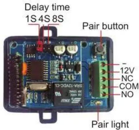
COM connections are same, Different are connected NO or NC.
