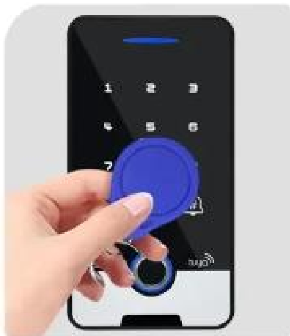
IC card swiping to open the door
