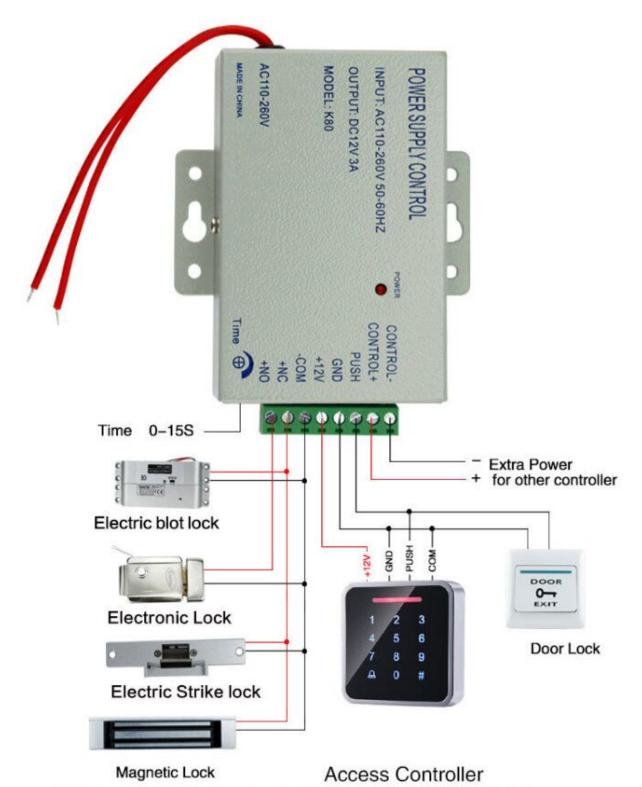
Attention when electronically contrlled lock must be transferred to 0seconds delay,to prevent burning of electric lock.
