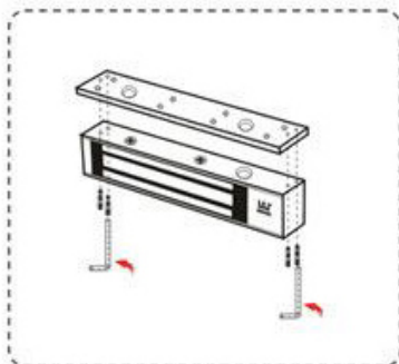
3. Separate the lock body and the connecting plate with a hexagonal key.
