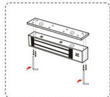
5. Secure the lock body and connecting plate with a hexagonal key.
