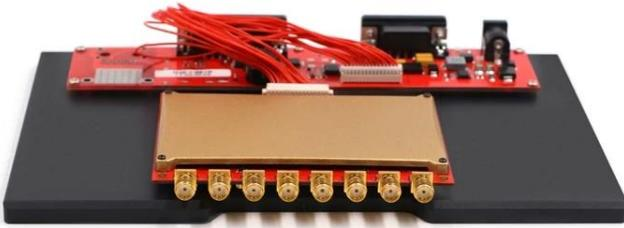
02 Module connect with antenna through SMA connector
