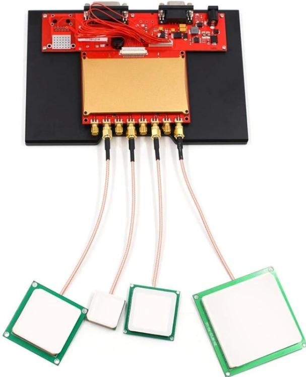
03 Interface board connect with power supply, use RS232 serial port connect with computer for communication, our interface board also with GPIO connector for option.
