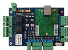
Network TCP/IP Access Control Board
