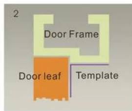
2 Close the door first, then place the upper side of template on door frame, while adjust the left side next to the door leaf.
