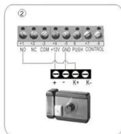
Attention! then electronically controlled lock must be transferred to 0 seconds delay, to prevent burning of electric locks.
