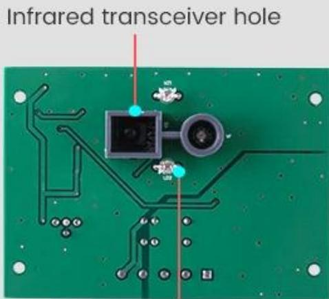
Infrared transceiver hole
