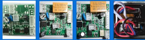
6 Wires PCB with timer 7 Wires PCB with timer and feedback 9 Wires PCB with timer and feedback Waterproof lock PCB
