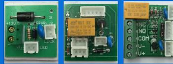
2 Wires PCB 5 Wires PCB with feedback function 12V/24V 5 Wires PCB with feedback function
