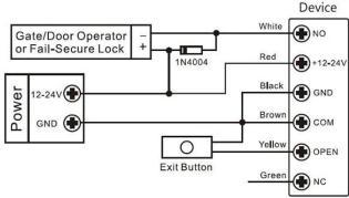
Attention: Install a 1N4004 or equivalent diode is needed when use a common power supply, or the reader might be damaged. (1N4004 is in cluded in the packing)
