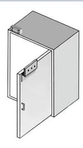
Demonstration of Z Bracket Installation
