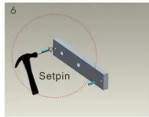
6 Strike the pin into the armature plate slightly (to avoid movement).
