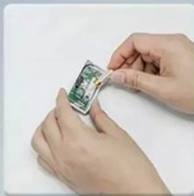
② install 23A 12V battery
