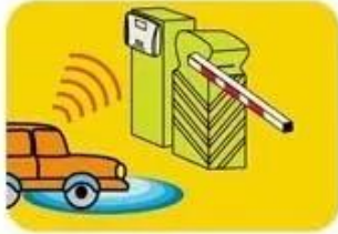
Vehicle access control system
