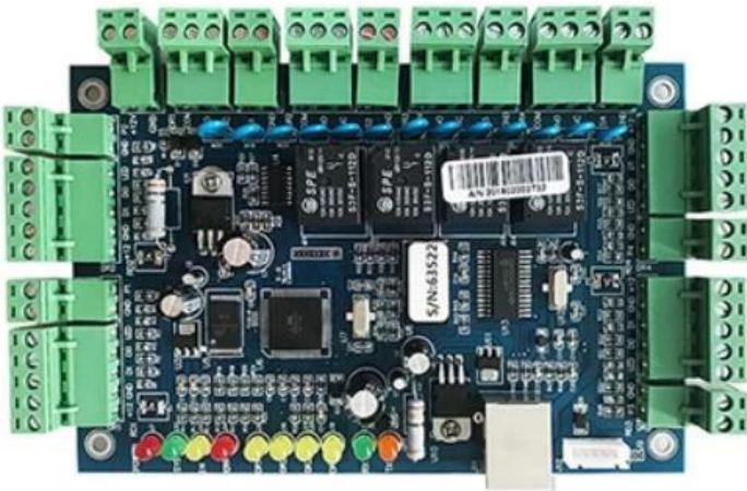
ACM-T04 > Four-door TCP/IP Network Door Controller
