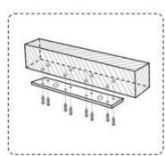
4.Find the appropriate position and attach the connecting plate to the door frame.
