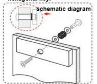
6.Install the attachment plate, first pad the gasket and rubber ring, and arrange them in order.
