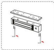
3. Separate the lock body and the the connecting plate with a hexagonal key.
