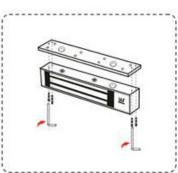
5.Secure the lock body and connecting plate with a hexagonal key.
