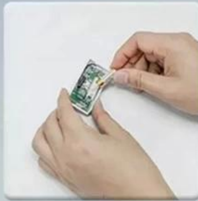
② install 23A 12V battery
