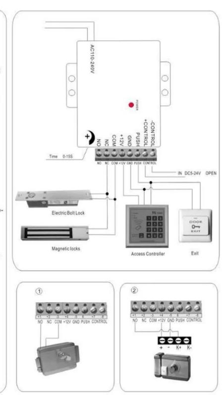
Attention! then electronically controlled lock must be transferred to 0 seconds delay, to prevent burning of electric locks.
