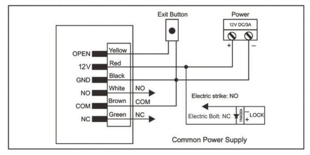
Attention: Install a 1N4004 or equivalent diode is needed when use a common power supply, or the keypad might be damaged. (1N4004 is included in the packing)
