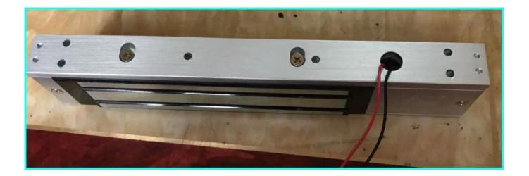
Our lock is with LED light to show the working statue , light is green when it locked , Red when unlocked . The light statue can be changed .
